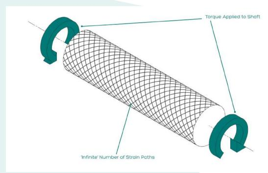
Datum Electronics Torque Transducers utilise this shaft bending and measure the change in order to calculate the torque. This measurement is achieved by the use of strain gauges bonded to the shaft, measuring the strain, induced in the shaft by the applied torque or "force". There are various methods of measuring this twist through a shaft, but strain gauges are recognised as one of the most reliable methods if you have the expertise to achieve this.
