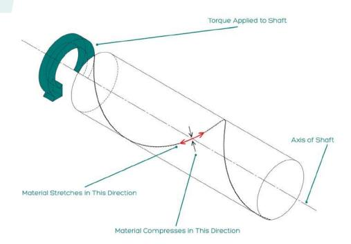
When a force of "torque" is applied to a shaft, the shaft twists (by a very small amount). This twisting produces a "stretch" in the material of the shaft, in a direction at 45 degrees to the axis of the shaft, between points on the shaft that are moved apart by the twisting motion. The material of the shaft also sees a "compression" in the opposite 45-degree direction.
