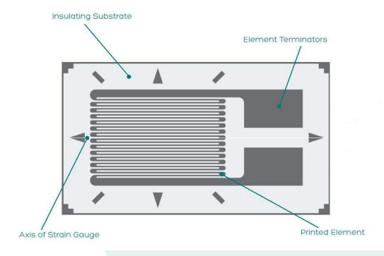
If a gauge is bonded to the shaft, with its axis aligned with the direction in which the shaft material stretches when a torque is applied, the strain gauge will also stretch and therefore the element will increase in resistance.
